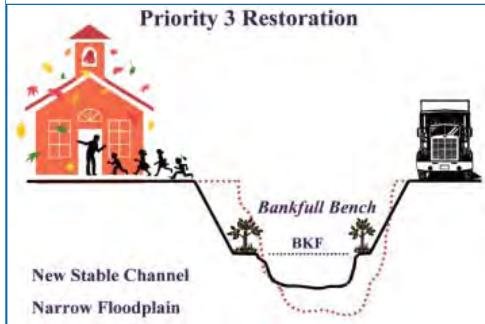
Figure 5.4 Cross section of a Priority 3 restoration project
