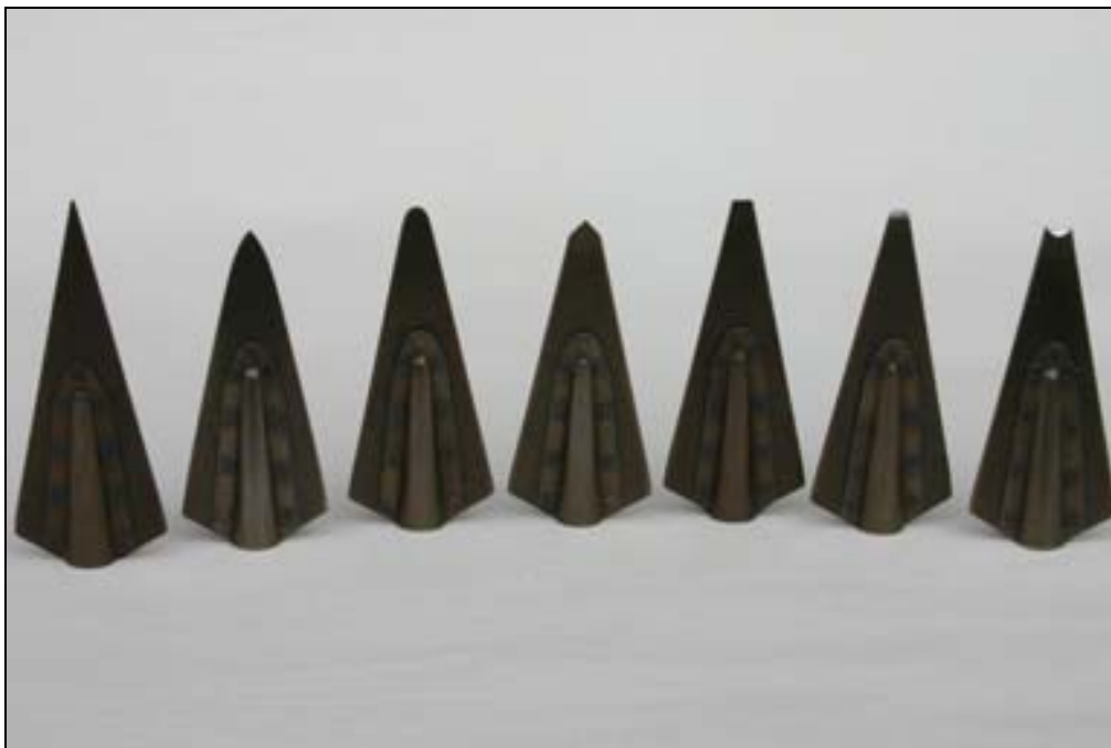
Tip designs tested included, from Left: Original Needle Tip; COI Arch; COI Round; COI Tanto; Flat; COI Chisel (flat); and COI Concave
