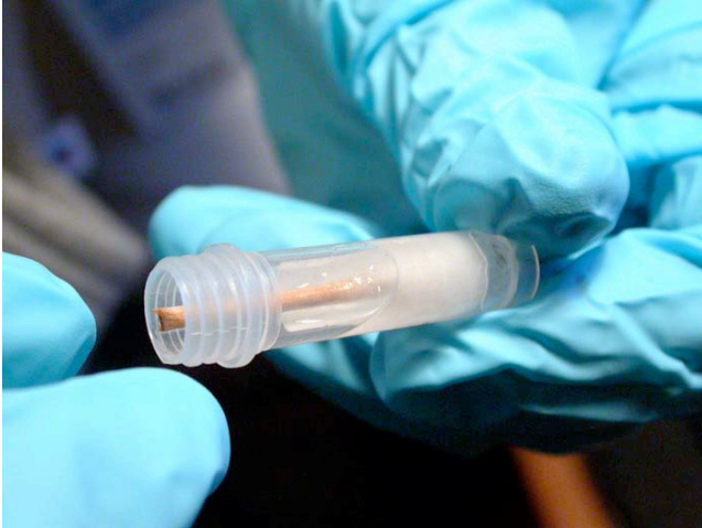
FIGURE 2. Insert swab or stick into tube with sample at bottom of tube.
