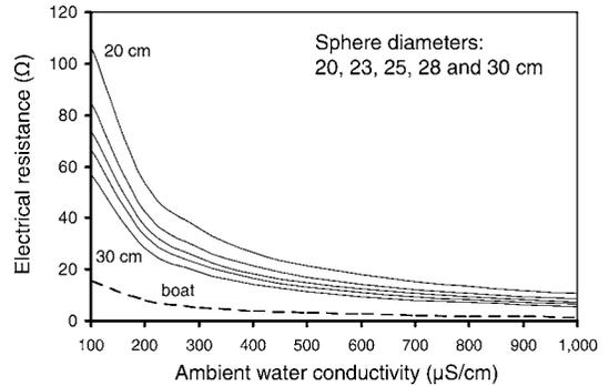
FIGURE 1.—Extrapolated electrofishing system resistance, including a 5.5-m aluminum-hulled, flat-bottom boat used as the cathode and two half-submerged pairs of stainless steel spherical anodes 20, 23, 25, 28, and 30 cm in diameter, at water conductivities ranging from 100 to 1,000  $\mu\text{S}/\text{cm}$ . The dotted line denotes the estimated resistance of the boat hull.
