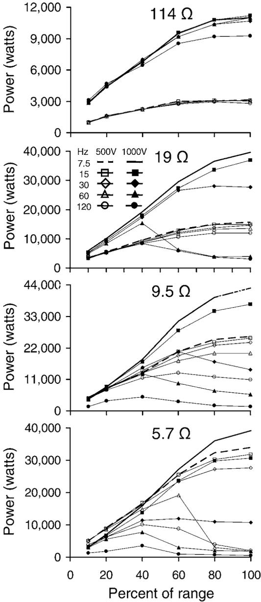
FIGURE 2.—Peak power output for Smith-Root GPP 5.0 electrofishers connected to static loads to simulate electrofishing electrodes in ambient water conductivities of 100, 400, 700, and 1,000  $\mu\text{S}/\text{cm}$ .
