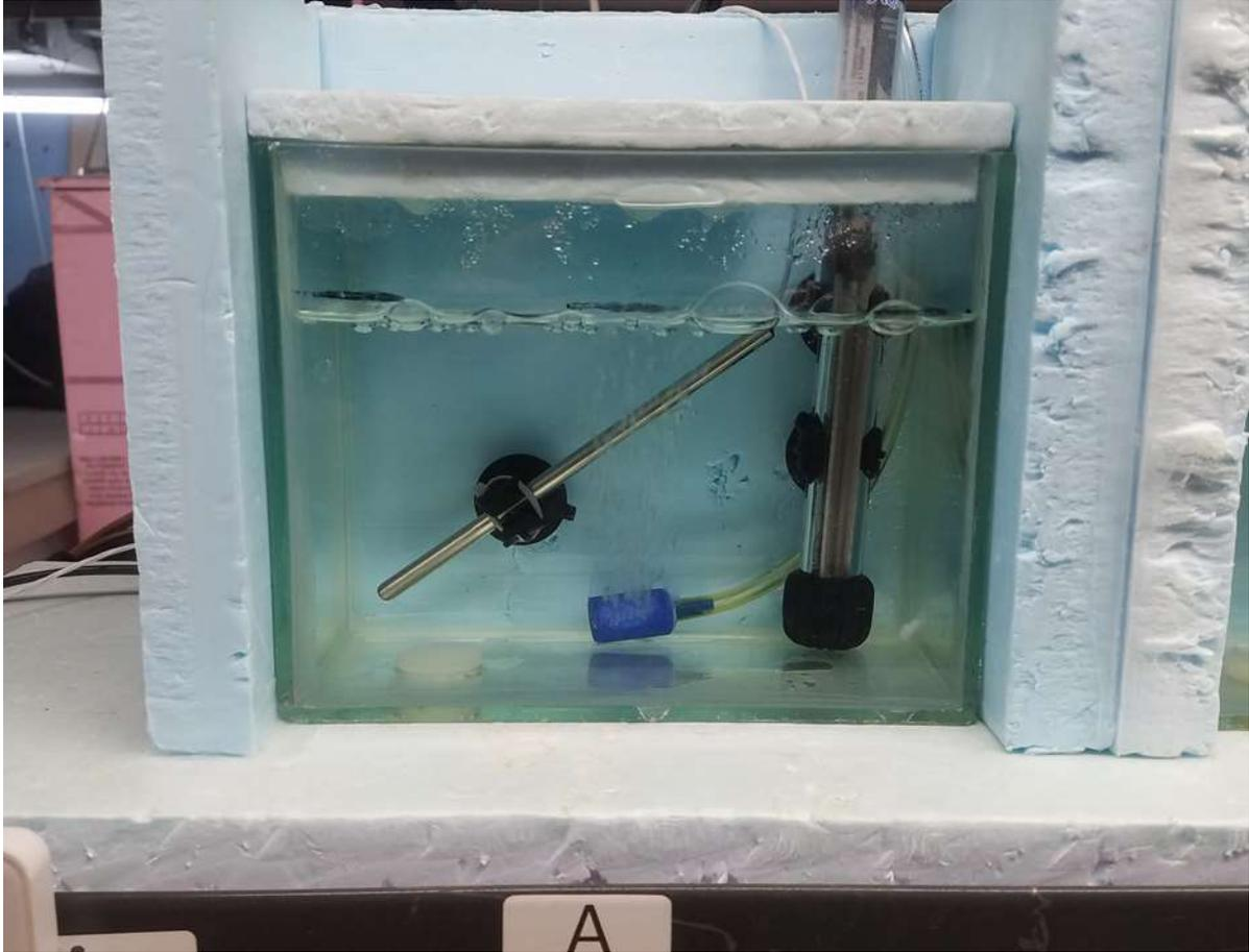
**Figure B3.** Critical thermal maxima (CTM) test tank. Fish were placed in the test tanks at their holding temperature (10°C). After an acclimation period the temperature was increased 0.3 °C/min until the fish displayed sustained loss of equilibrium. Love Controls series 16b temperature controllers fitted with titanium heat probes and 100w aquarium heaters were programmed to adjust the temperature. Dissolved oxygen levels were held constant throughout the test with an adjustable air stone.
