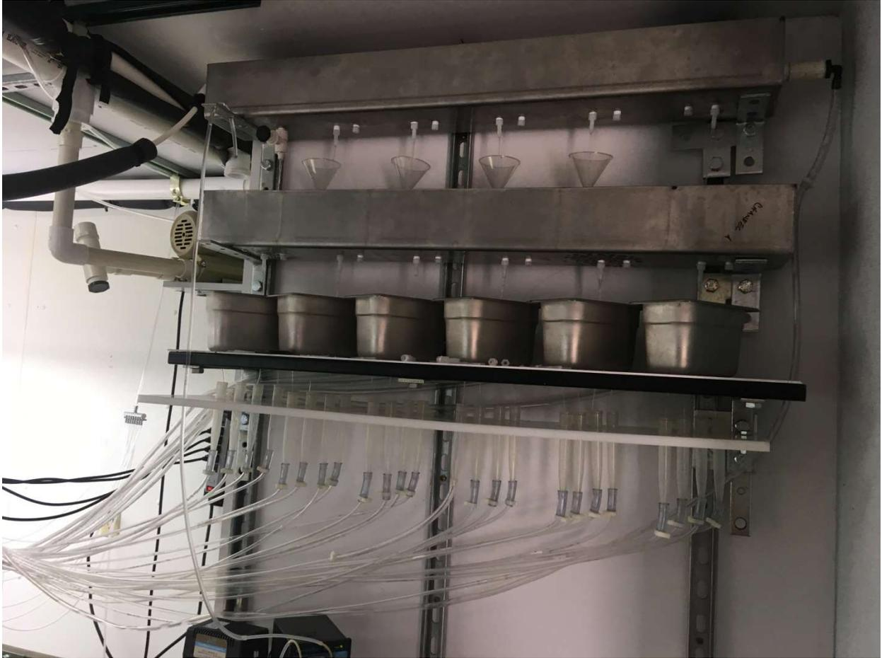
**Figure A2.** Gravity-fed serial diluter.
