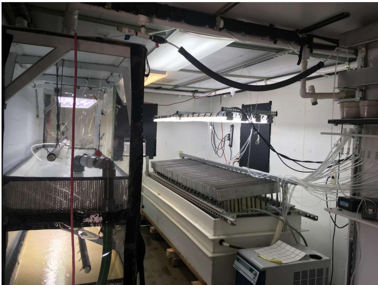
**Figure A3.** Algal culture systems (left) delivered a slow supply to the serial toxicant diluter (right) which delivered toxicants and dechlorinated water to the twenty-four experiment streams in a chilled water bath (center).
