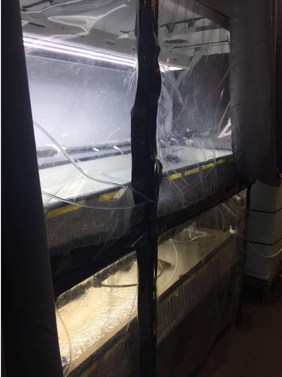
**Figure A1.** Algal culture system. Two chilled water baths received flow-through dechlorinated municipal water at a 95% replenishment rate of 18 hours. Additionally baths recirculated into each other, had drippers and misters that kept cobble hydrated. Surfaces were disturbed daily and additional substrate (unglazed tiles) were added daily to ensure pioneer species were not out-competed during the experiment.
