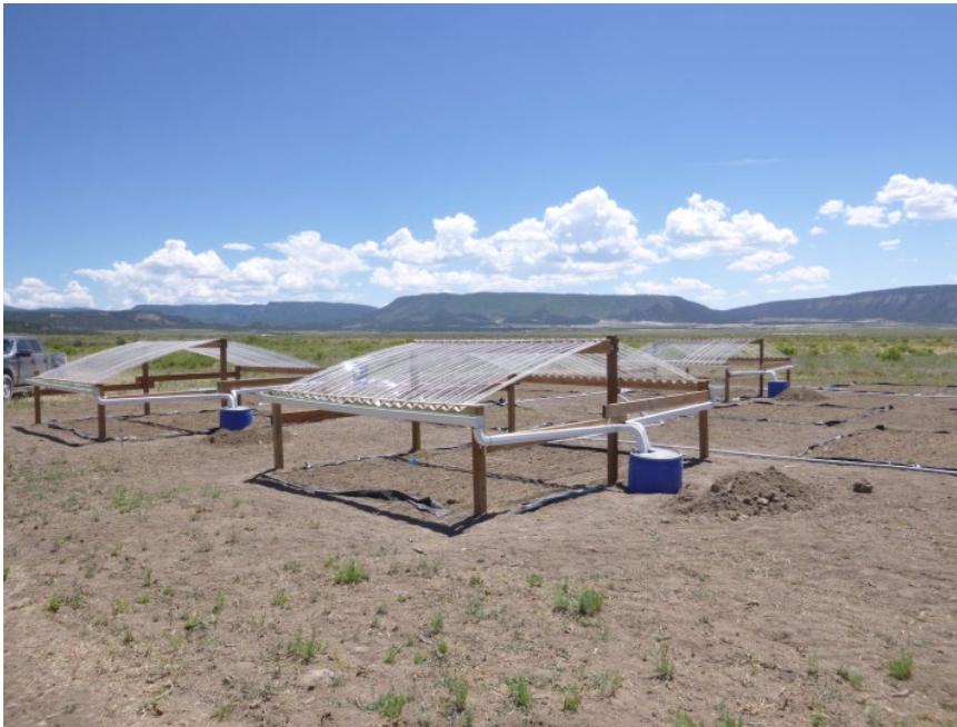
Figure 1. Rainfall exclusion shelters induce artificial drought at the Western Slope site in 2014.
