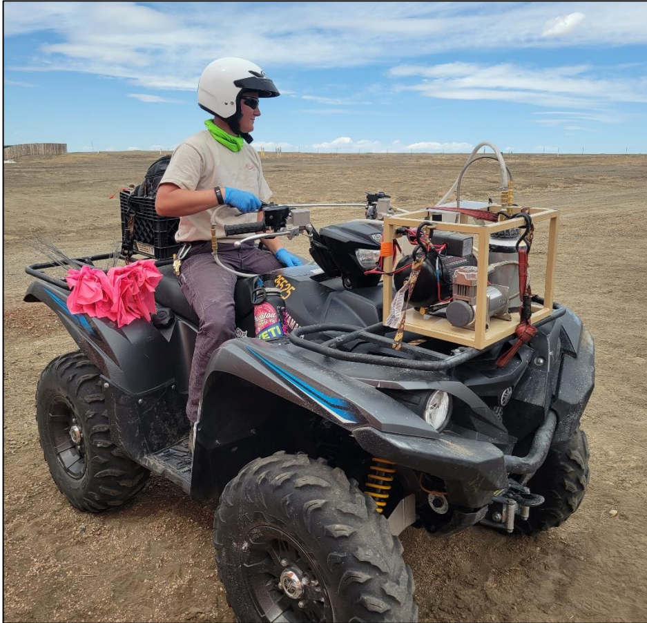
Figure 1. A low-pressure duster mounted on an ATV. The first six prototypes were field tested at Soapstone Prairie Natural Area in 2021.
