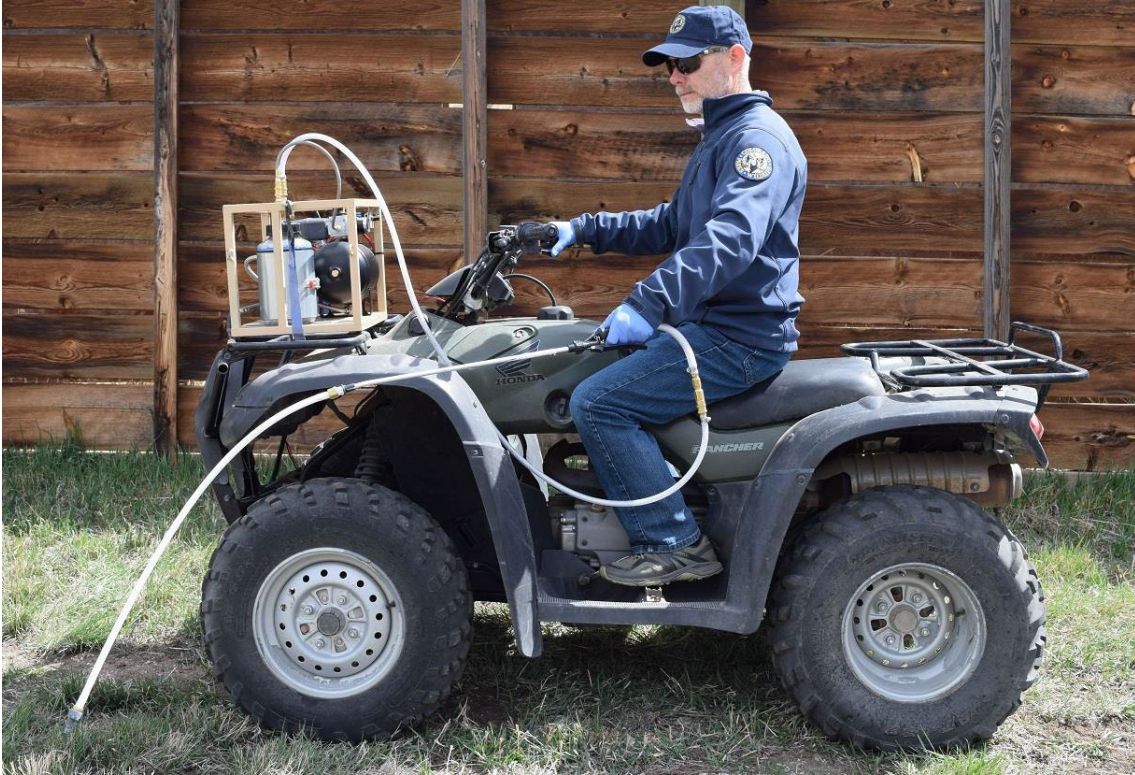
Figure 1. A low-pressure duster mounted on an ATV. The first six prototypes were field tested at Soapstone Prairie Natural Area in 2021.
