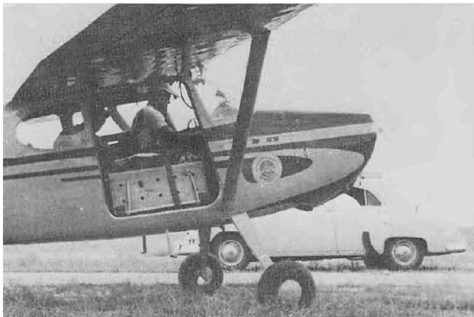
Figure 7-1. A Cessna 170 with the passenger door removed and a beaver parachute drop box ready for flight, during the CO Game and Fish Department experimental parachute beaver release in 1951.
