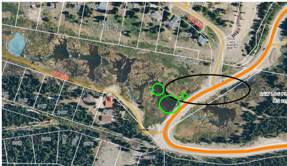
Figure 6-1. Photo provided by Summit County Open Space and Trails staff showing numerous beaver ponds on both sides of Highway 9 near Quandary Pass where a flow device (green circles) was successfully installed by Summit County. The black circle indicates where flooding of the road once occurred prior to the flow device being installed.
