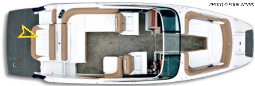
The engine motor compartment is located in the rear of the boat.
