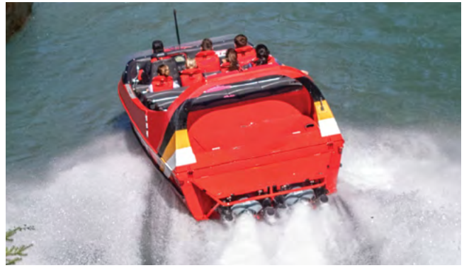
This jet stream exits through a small nozzle at high velocity to push the boat forward.
