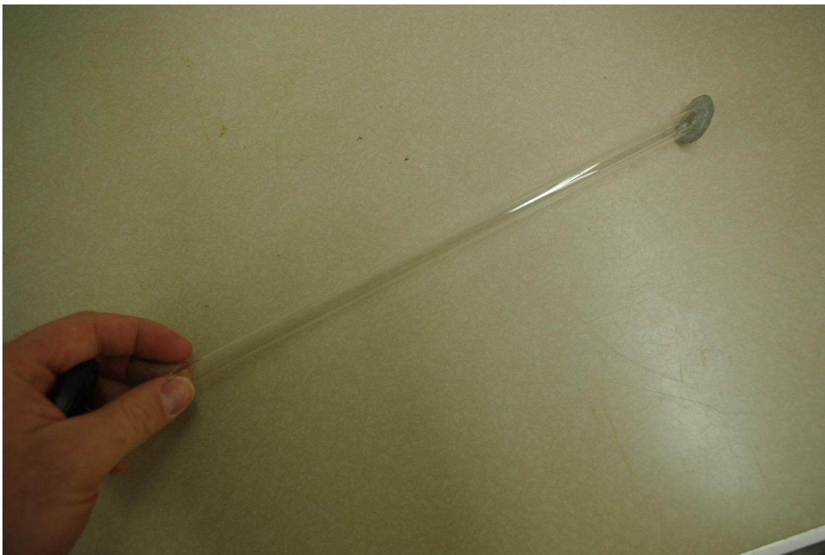
Figure 1.1.2-3. Borosilicate tubes (8mm ID, 12 mm OD) were used to house organisms during exposure and enumeration.
