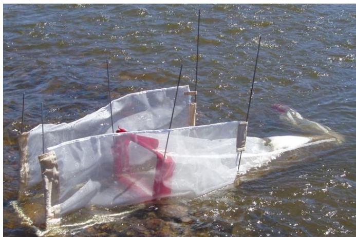
Figure 2: 0.25m 2 benthic sampling net used at all Windy Gap study sites.
