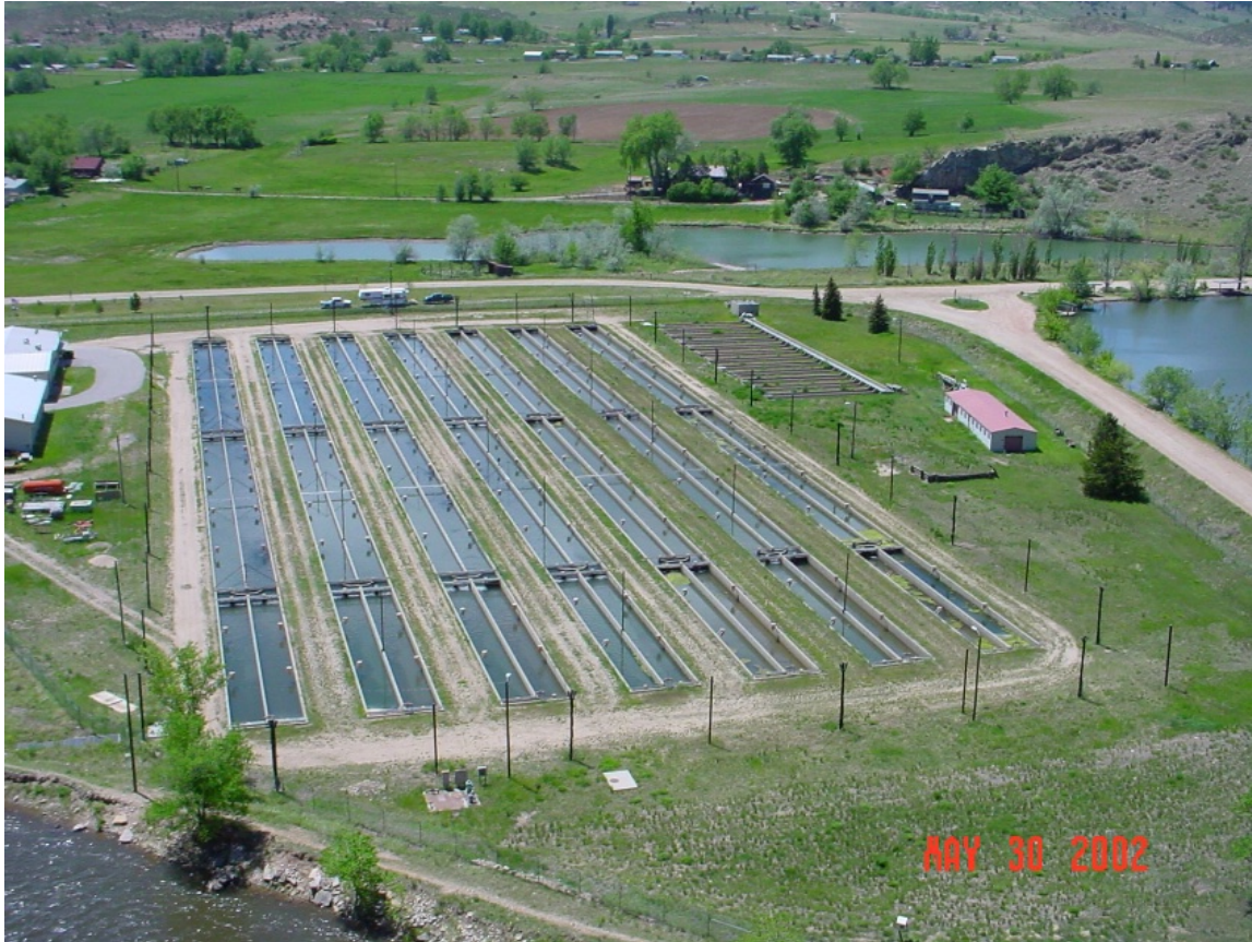
Figure A2.1. Watson hatchery uses surface water from the Cache la Poudre River, visible in bottom left corner. The water is diverted into a Watson Lake (visible to the right of the road on right side of picture) before coming into the raceways. We sampled fish from Watson that had previously resided at Bellevue, less than a mile away. Photo provided by Jim McKissick, CDOW.
