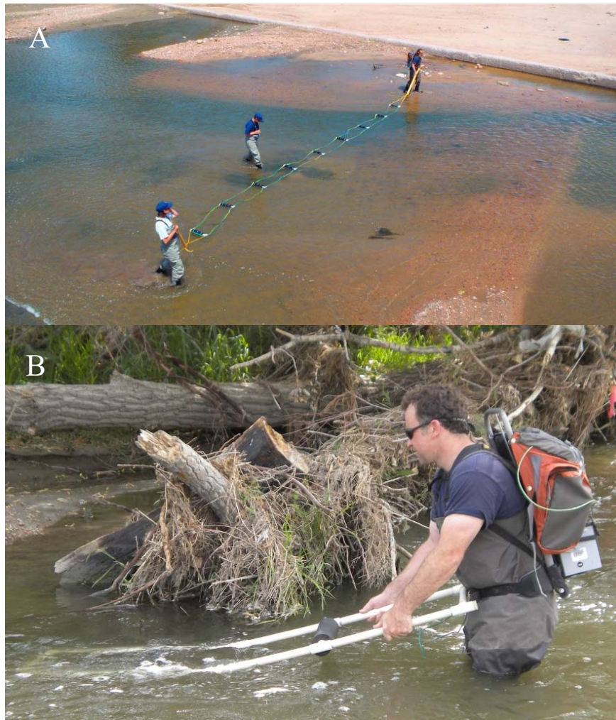
Figure 3. A. 12-m mobile array deployed at Owens Diversion. This array specialized in detecting tagged fish in the main channel. B. 2-m mobile array that was used to detect tagged fish in shoreline habitat.
