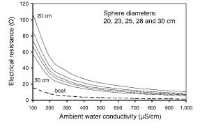
FIGURE 1.—Extrapolated electrofishing system resistance, including a 5.5-m aluminum-hulled, flat-bottom boat used as the cathode and two half-submerged pairs of stainless steel spherical anodes 20, 23, 25, 28, and 30 cm in diameter, at water conductivities ranging from 100 to 1,000  $\mu$ S/cm. The dotted line denotes the estimated resistance of the boat hull.
