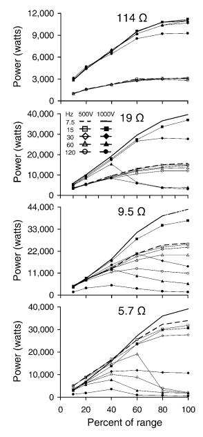
FIGURE 2.—Peak power output for Smith-Root GPP 5.0 electrofishers connected to static loads to simulate electrofishing electrodes in ambient water conductivities of 100, 400, 700, and 1,000  $\mu$ S/cm.
