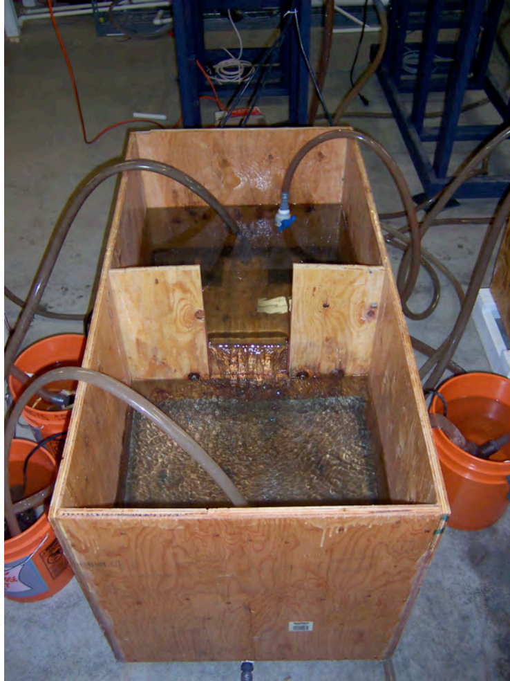
Figure 2.2 — A Kondratieff-type artificial waterfall used to test the jumping ability of small fishes. The orange buckets contain submersible pumps that pumped water from the lower chamber (bottom) into the upper chamber (top). The water then flowed over the weir back into the lower chamber.
