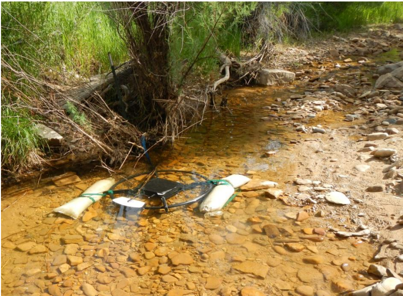
A small PIT tag antenna placed to detect spawning fish using a tributary stream
