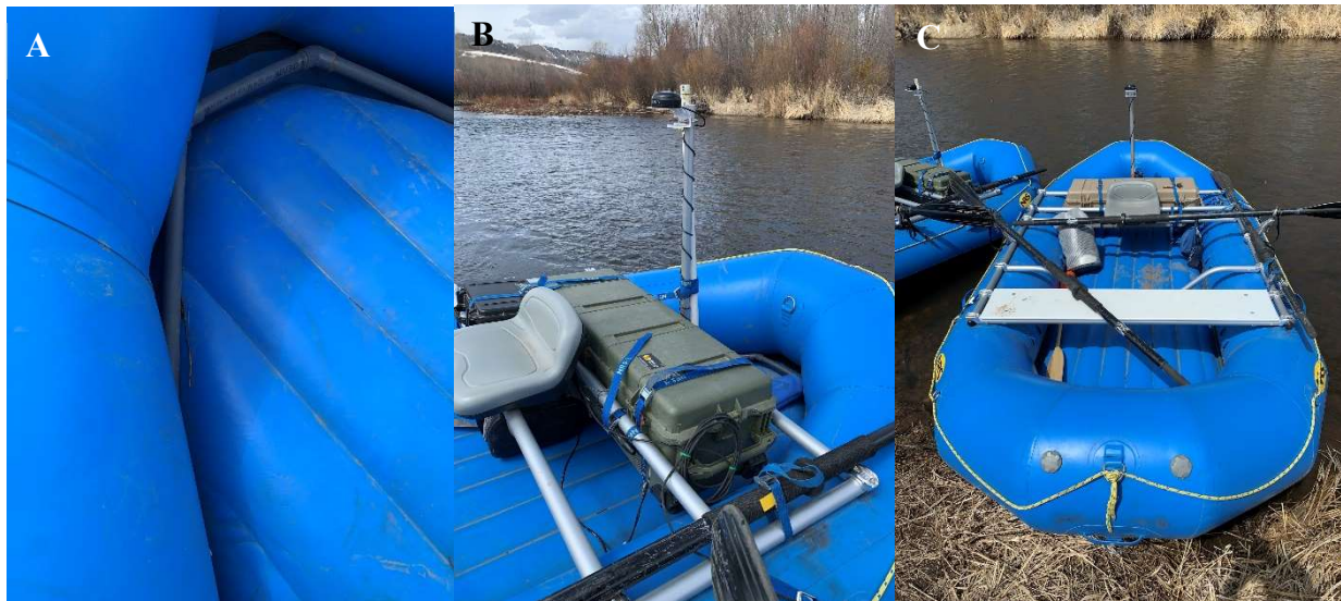
Figure 2.19. (A) Antenna wire encased in PVC to maintain rigidity, shape, and tuning during deployment. (B) Pelican box, containing batteries, reader, tuner box, and Campbell Scientific datalogger, and external GPS unit for marking the location of detected PIT tags. (C) Portable antennas set to deploy on the Fraser River Ranch.
