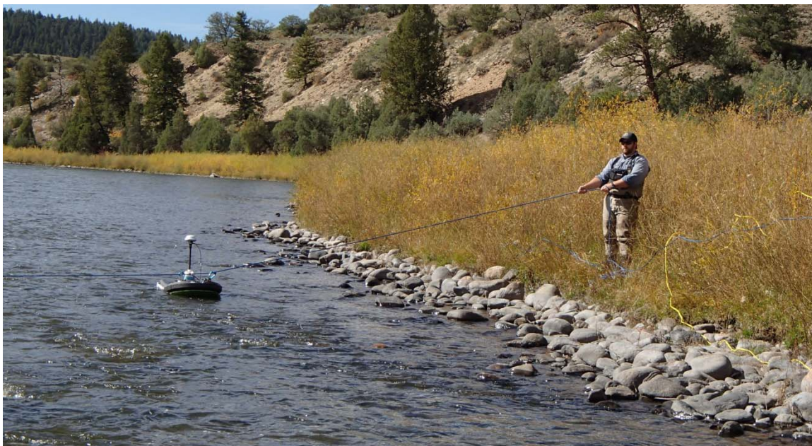
Figure 2.1 Surveying riffle morphology with the SonTek ADCP HydroSurveyor on the Colorado River near Pumphouse.
