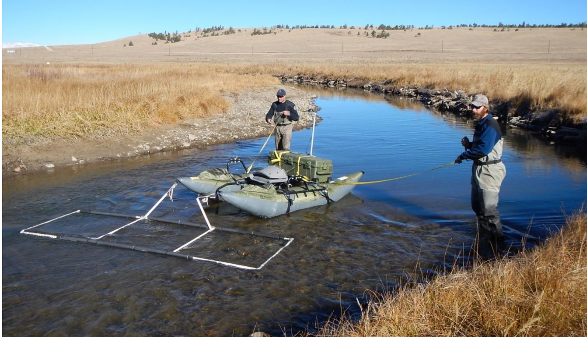
Figure 3.1. Deployment of the RFID-GPS system on the Middle Fork South Platte River.
