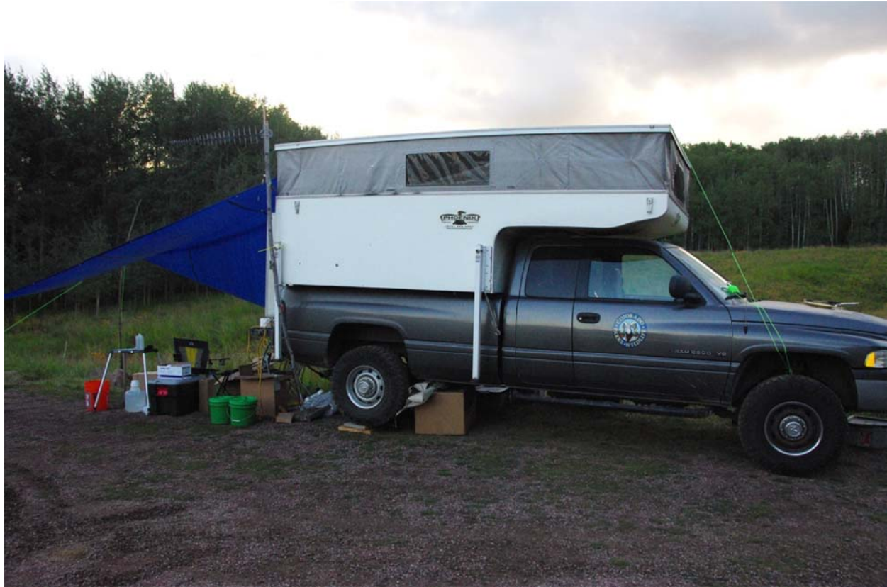
Figure 2.1 – Mobile Laboratory. Our analytical service is often located next to detox (the MnO_4 drip station used in lotic reclamation projects) because this is typically where the majority of samples are taken. Some of the detox stations in Colorado were assembled using pack mules or helicopters. Trailers were often difficult to maneuver on Colorado’s rough ‘Jeep trails.’ Sample preparation was done outside and space was limited, However, this system allowed off-road ability, a dry location for the instrument.
