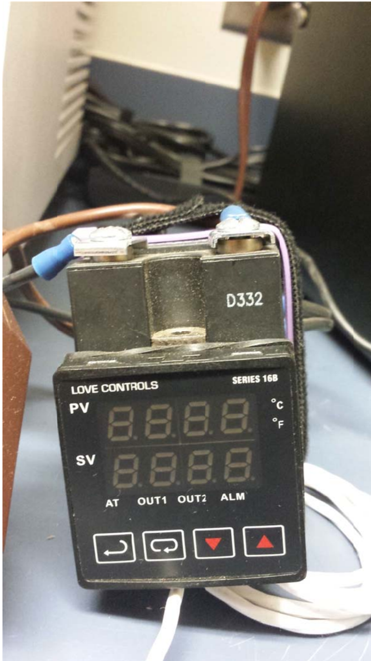
Figure 2.16- Love 16B temperature controller.
