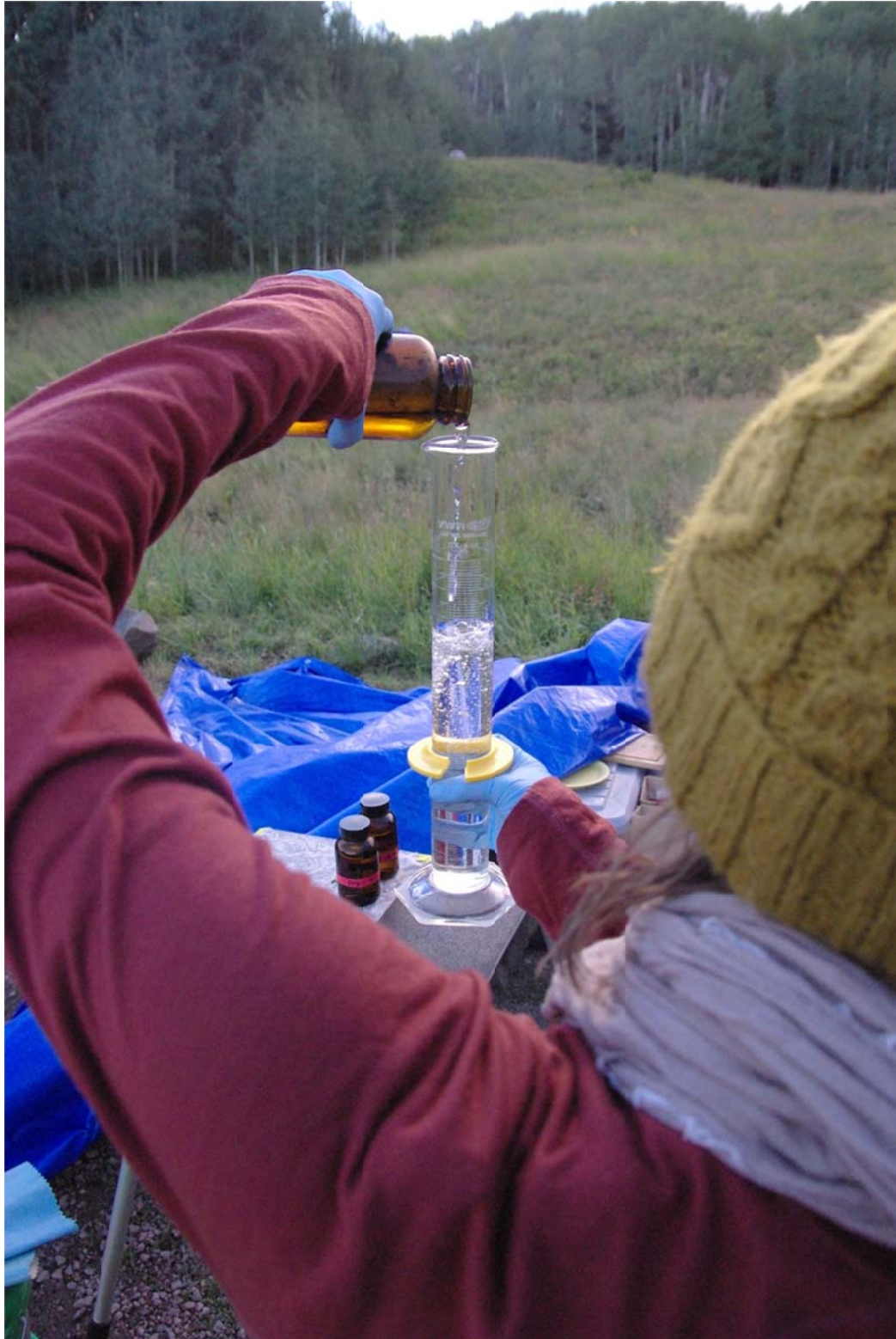
Figure 2.6 – Samples were measuring to 200ml in a graduated cylinder.
