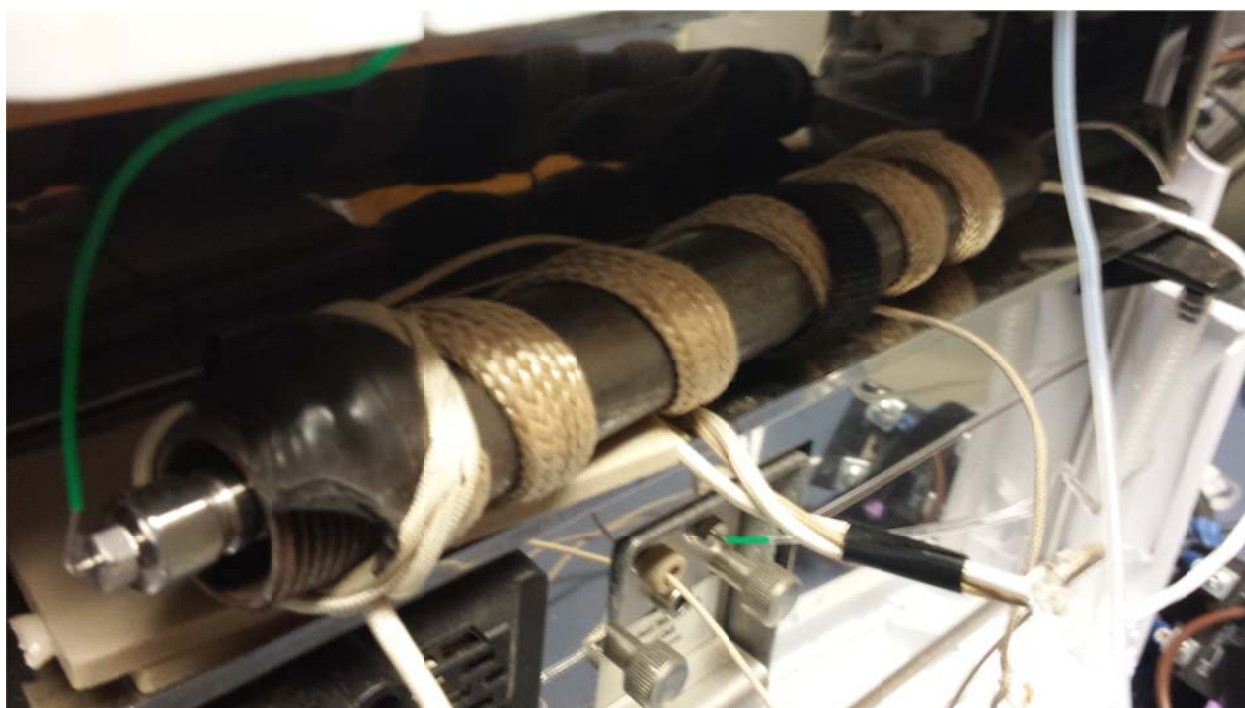
Figure 2.14- Pipe with heat tape and Love temperature controller. The HPLC column and thermometer for the temperature controller were placed in the steel pipe.
