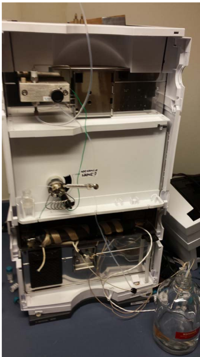
Figure 2.13 – Agilent 1220 HPLC with column hidden in a heating system consisting of a 6 inch piece of steel pipe, pipe heat tape, and a temperature controller.
