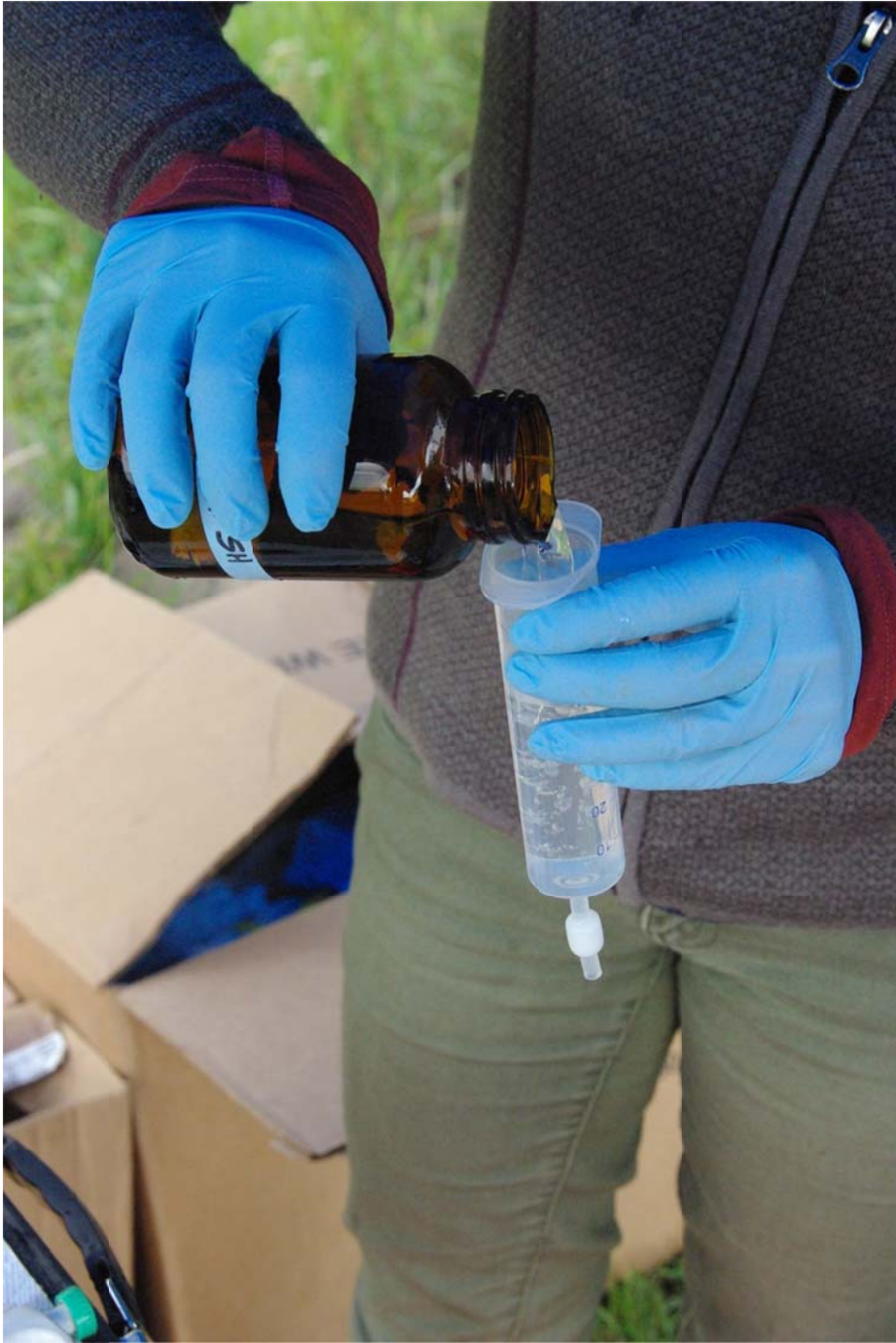
Figure 2.9 – The 60ml syringe was loaded from the back end.
