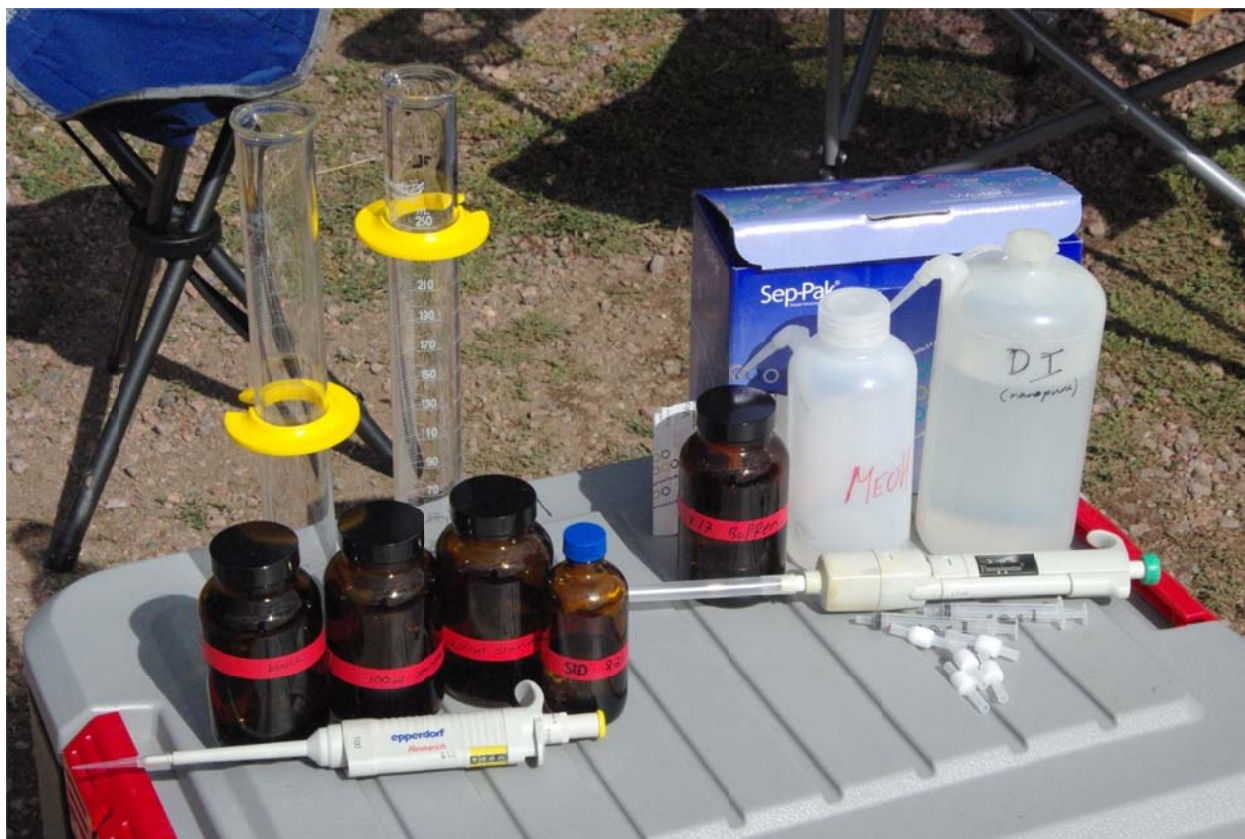
Figure 2.8- Equipment used in extractions, sample preparation, and making a standard curve. Left to right: 100µl pipette, 3 sample bottles (250ml) used to create a calibration curve, 1 glass amber (125ml) containing the rotenone standard, 250ml graduated cylinders, 1-5ml adjustable pipette, 5 Sep-Pak cartridges and 3ml syringes, squirt bottles of methanol and DI water.
