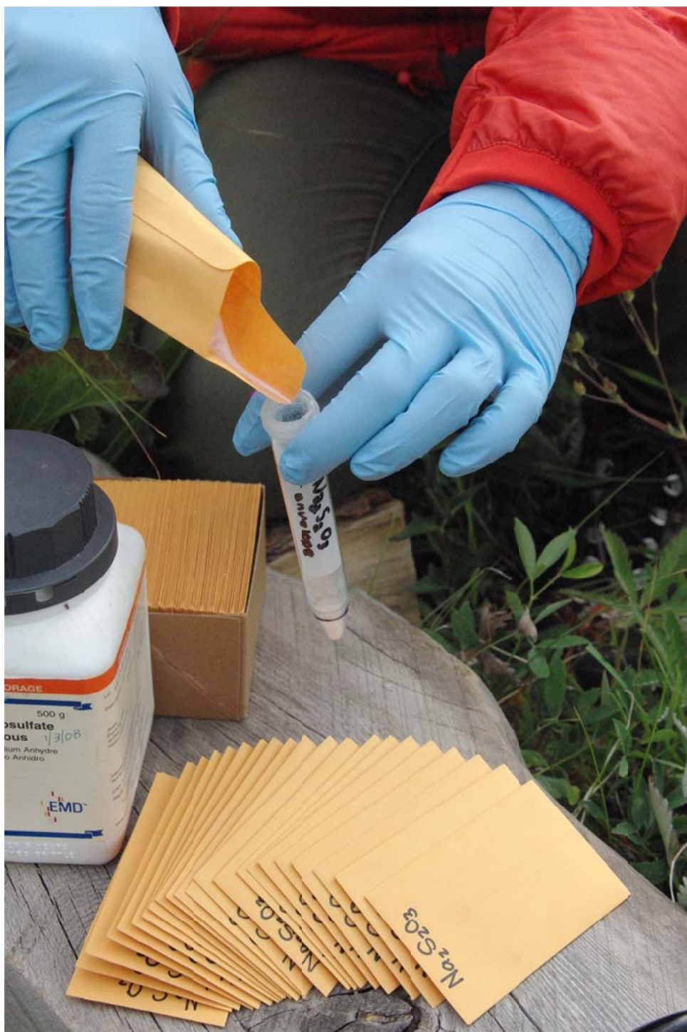
Figure 2.4 – Sodium thiosulfate preservative. A graduated centrifuge tube was used to measure ~0.25ml of Sodium thiosulfate which was sealed in a disposable coin envelope. This substance prevented the decay of rotenone in samples. The mass of this solid is in excess of what is needed to neutralize \text{KMnO}_4 , thus precision was not needed.
