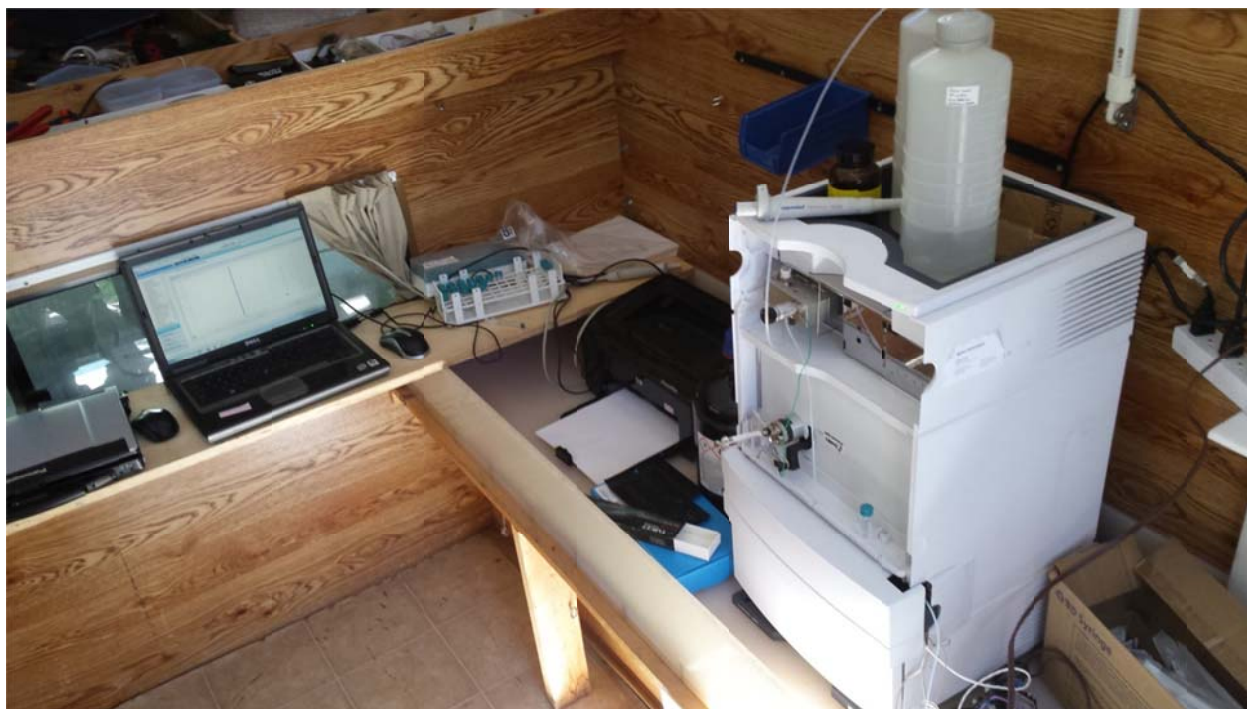
Figure 2.12 – HPLC, laptop and printer. Photo from inside the mobile laboratory showing the Agilent 1220.
