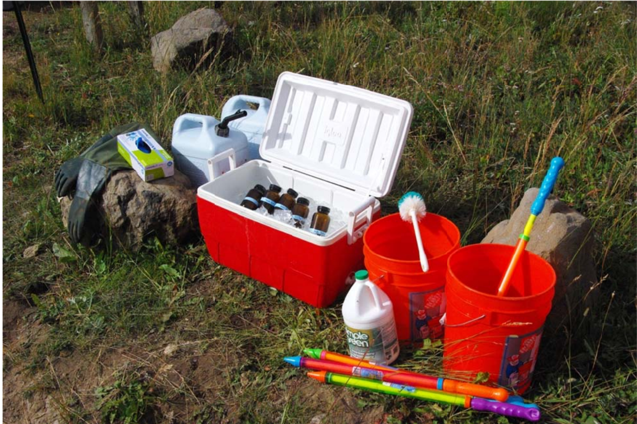
Figure 2.5- Sample decontamination station. Decontamination of sample bottles and keeping wader clad field staff from the preparation area reduced contamination issues in sample preparation and analysis. The wash station included buckets with rinse water and mild detergent (Simple Green), scrub brushes, water squirters or pressurized sprayers, personal protective equipment and an ice chest.
