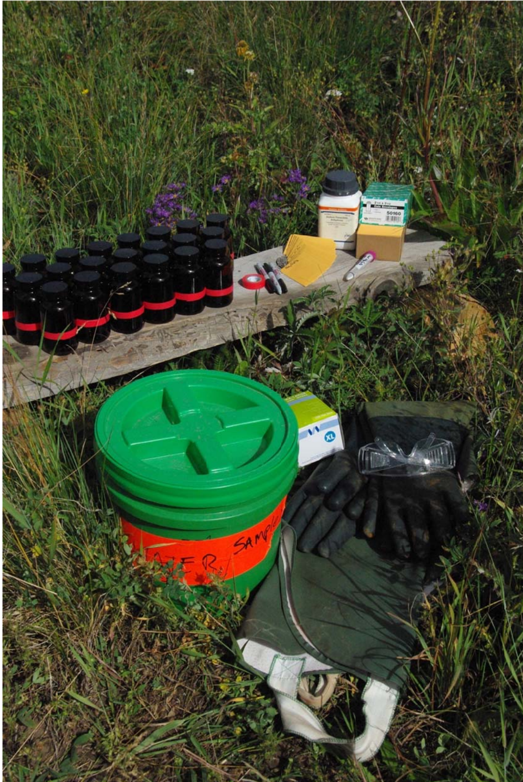
Figure 2.3 – Field collection equipment station. Every morning bottles, envelopes of preservative, small coolers (bucket) and PPE were made available to field staff responsible for collecting samples.
