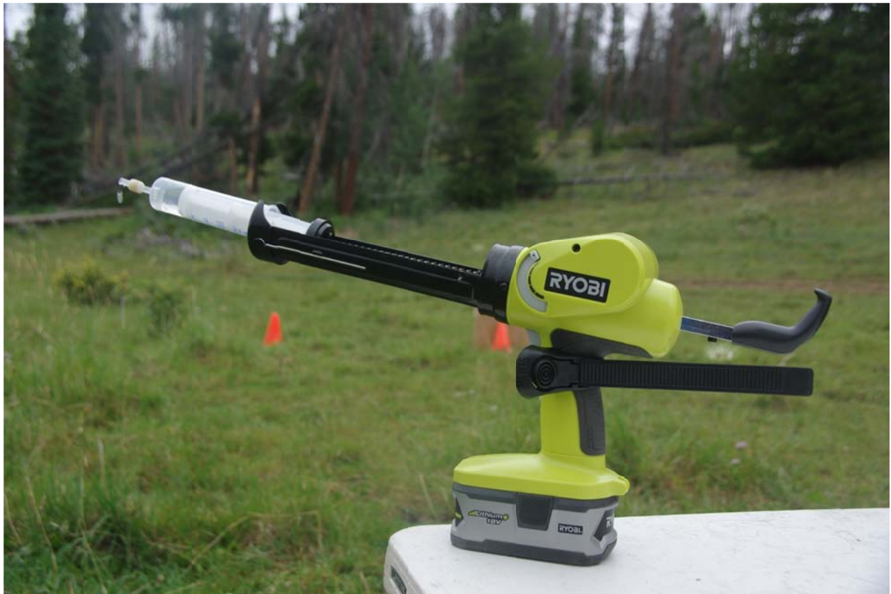
Figure 2.11- Battery powered caulk gun. These caulk guns ($40) were far more reliable in the field than laboratory syringe pumps ($1200-3000).
