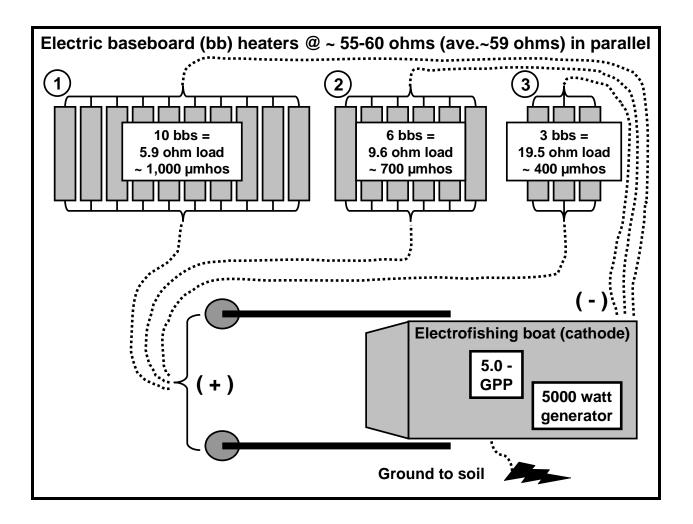
**Figure 5.** Diagram of set-up for subjecting a Smith-Root Model 5.0-GPP electrofisher to three levels of electrical resistance, 1) 5.9, 2) 9.6, and 3) 19.5 ohms, by using varying arrays of baseboard heaters to simulate water conductivities of 1,000, 700, and 400 μmhos, respectively.
