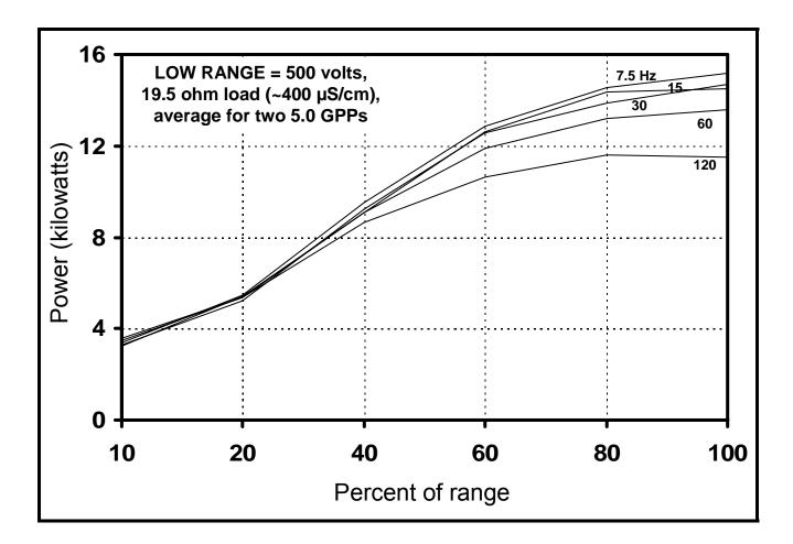
**Figure 9.** Power output for Smith-Root Model 5.0 GPP electrofisher, averaged for two units, operating at the LOW RANGE 500 volt setting in the DC mode (Figure 1). Electrofishers were subjected to an electrical load of 19.5 ohms simulating an approximate water conductivity of 400  $\mu$ S/cm, as illustrated in Figure 3, and operated at percent of range settings of 10, 20, 40, 60, 80 and 100 at pulse per second settings of 7.5, 15, 30, 60 and 120 Hz.
