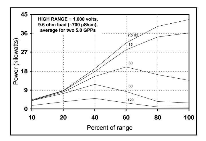
**Figure 14.** Power output for Smith-Root Model 5.0 GPP electrofisher, averaged for two units, operating at the HIGH RANGE 1,000 volt setting in the DC mode (Figure 1). Electrofishers were subjected to an electrical load of 9.6 ohms simulating an approximate water conductivity of 700  $\mu$ S/cm, as illustrated in Figure 3, and operated at percent of range settings of 10, 20, 40, 60, 80 and 100 at pulse per second settings of 7.5, 15, 30, 60 and 120 Hz.
