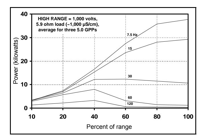
**Figure 15.** Power output for Smith-Root Model 5.0 GPP electrofisher, averaged for three units, operating at the HIGH RANGE 1,000 volt setting in the DC mode (Figure 1). Electrofishers were subjected to an electrical load of 5.9 ohms simulating an approximate water conductivity of 1,000  $\mu$ S/cm, as illustrated in Figure 3, and operated at percent of range settings of 10, 20, 40, 60, 80 and 100 at pulse per second settings of 7.5, 15, 30, 60 and 120 Hz.
