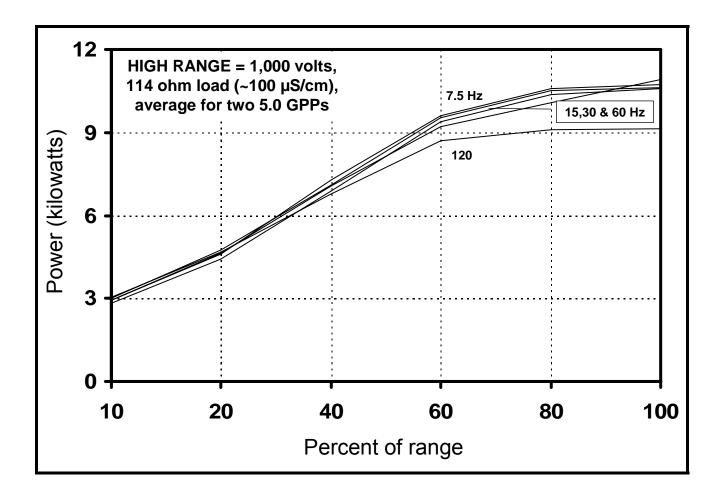
**Figure 12.** Power output for Smith-Root Model 5.0 GPP electrofisher, averaged for two units, operating at the HIGH RANGE 1,000 volt setting in the DC mode (Figure 1). Electrofishers were subjected to an electrical load of 114 ohms simulating an approximate water conductivity of 100  $\mu$ S/cm, as illustrated in Figure 4, and operated at percent of range settings of 10, 20, 40, 60, 80 and 100 at pulse per second settings of 7.5, 15, 30, 60 and 120 Hz.
