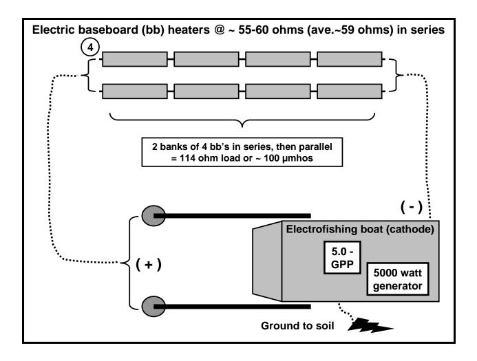
**Figure 6.** Diagram of set-up for subjecting a Smith-Root Model 5.0-GPP electrofisher to a fourth level of electrical resistance of 114 ohms using two arrays of four baseboard heaters in series, then parallel, to simulate a water conductivity of 100 µmhos.
