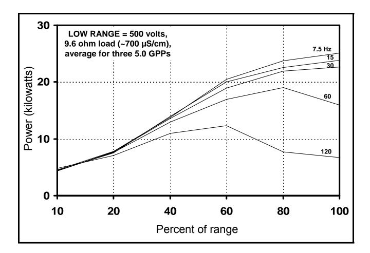
Figure 10. Power output for Smith-Root Model 5.0 GPP electrofisher, averaged for three units, operating at the LOW RANGE 500 volt setting in the DC mode (Figure 1). Electrofishers were subjected to an electrical load of 9.6 ohms simulating an approximate water conductivity of 700  $\mu$ S/cm, as illustrated in Figure 3, and operated at percent of range settings of 10, 20, 40, 60, 80 and 100 at pulse per second settings of 7.5, 15, 30, 60 and 120 Hz.
