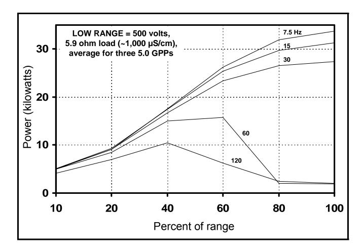
**Figure 11.** Power output for Smith-Root Model 5.0 GPP electrofisher, averaged for three units, operating at the LOW RANGE 500 volt setting in the DC mode (Figure 1). Electrofishers were subjected to an electrical load of 5.9 ohms simulating an approximate water conductivity of 1,000  $\mu$ S/cm, as illustrated in Figure 3, and operated at percent of range settings of 10, 20, 40, 60, 80 and 100 at pulse per second settings of 7.5, 15, 30, 60 and 120 Hz.
