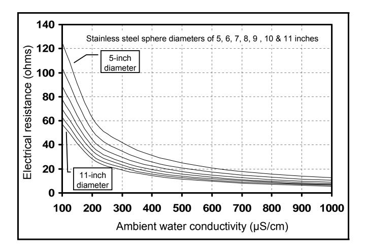
**Figure 4.** Theoretical electrical resistance of stainless steel spheres of 5, 6, 7, 8, 9, 10, and 11 inches in diameter at water conductivities ranging from 100 to  $1000 \,\mu$ S/cm.
