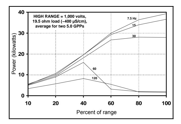
**Figure 13.** Power output for Smith-Root Model 5.0 GPP electrofisher, averaged for two units, operating at the HIGH RANGE 1,000 volt setting in the DC mode (Figure 1). Electrofishers were subjected to an electrical load of 19.5 ohms simulating an approximate water conductivity of 400  $\mu$ S/cm, as illustrated in Figure 3, and operated at percent of range settings of 10, 20, 40, 60, 80 and 100 at pulse per second settings of 7.5, 15, 30, 60 and 120 Hz.
