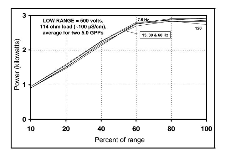
**Figure 8.** Power output for Smith-Root Model 5.0 GPP electrofisher, averaged for two units, operating at the LOW RANGE 500 volt setting in the DC mode (Figure 1). Electrofishers were subjected to an electrical load of 114 ohms simulating an approximate water conductivity of 100  $\mu$ S/cm, as illustrated in Figure 4, and operated at percent of range settings of 10, 20, 40, 60, 80 and 100 at pulse per second settings of 7.5, 15, 30, 60 and 120 Hz.
