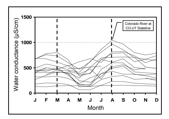
**Figure 2.** Ambient conductivity ( $\mu$ S/cm) at 16 stream gage stations in western Colorado, 1997-2005 (see Figure 1). Vertical dashed lines delineate the five-month period from March through July, the time of year when stream flows permit widespread use of aluminum-hulled electrofishing boats in rivers of the Upper Colorado River Basin. The mean monthly ambient conductivity in July in the Colorado River at Colorado-Utah Stateline is the only gage to exceed 1000  $\mu$ S/cm.
