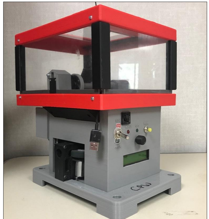
Figure 61. Side view of 3-shooter. Baits will fall from the center and bounce off the fender of ATV.
