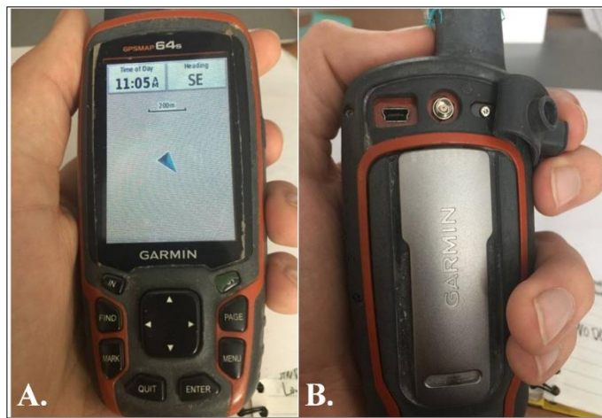
Figure 9. Garmin 64s GPS unit. A. Front of unit turned on and displaying the MAP window. B. Back of unit with USB port exposed.
