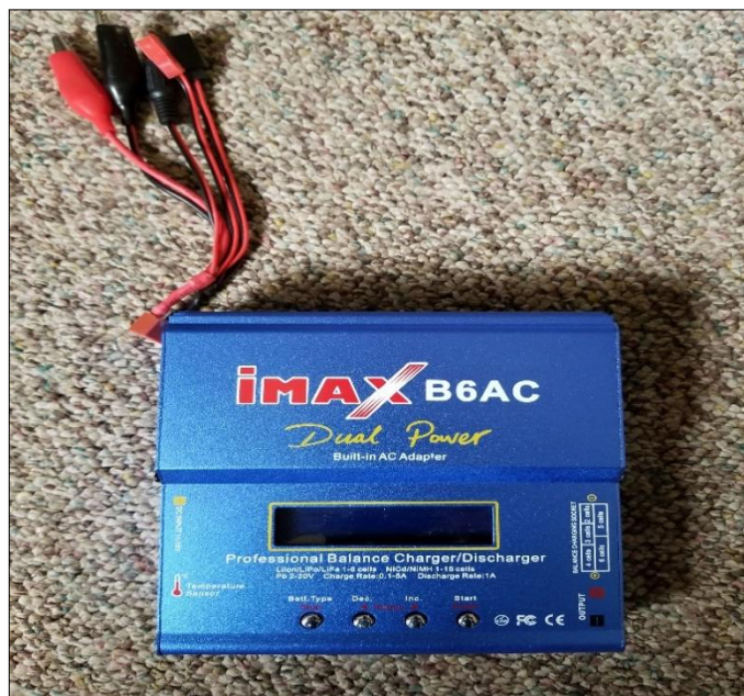
Figure 63. Imax B6AC Lithium Polymer (LiPo) 3-shooter battery charger.
