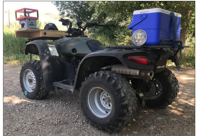
Figure 60. ATV ready for bait distribution. Cooler and three shooter strapped down securely and GPS mounted to handlebars.
